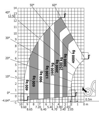
Machine on lowered stabilisers with forks Metric
